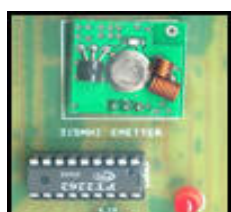
RF TRANSMITTER USING 2262 Encoder ic.
